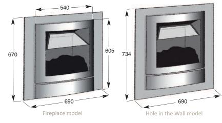
Measurements of visible parts only are shown. For further measurements please see page 31.
