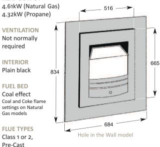
Measurements of visible parts only are shown. For further measurements or for fireplace model see page 35.
