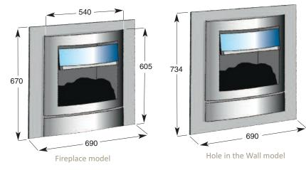
Measurements of visible parts only are shown. For further measurements please see page 27.
