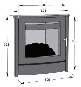
Measurements of visible parts only are shown. For further measurements please see page 41.
